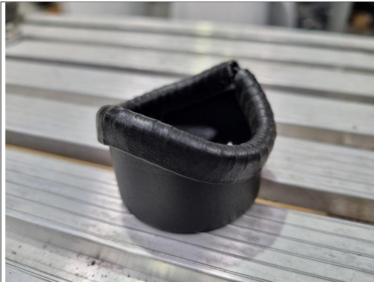
25. Fit supplied pinch weld around the curved edge of the spigot. Trim with side cutters as required.
