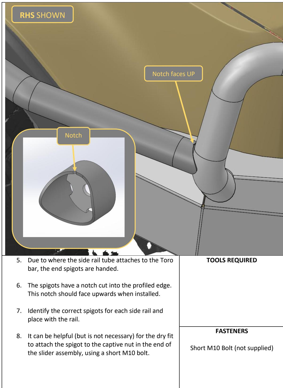
5. Due to where the side rail tube attaches to the Toro bar, the end spigots are handed.
