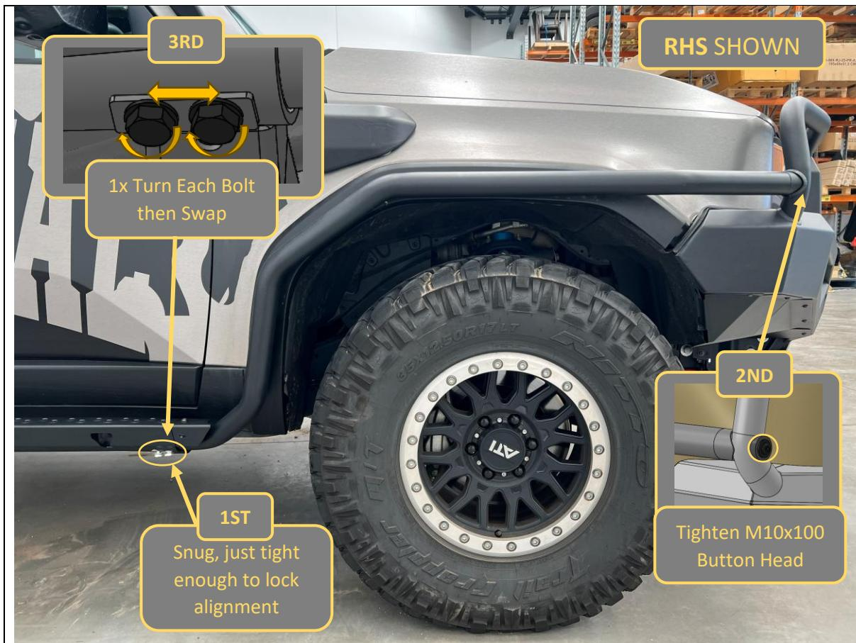
27. Refit the scrub rail to the rock slider, using the same procedure as earlier.
